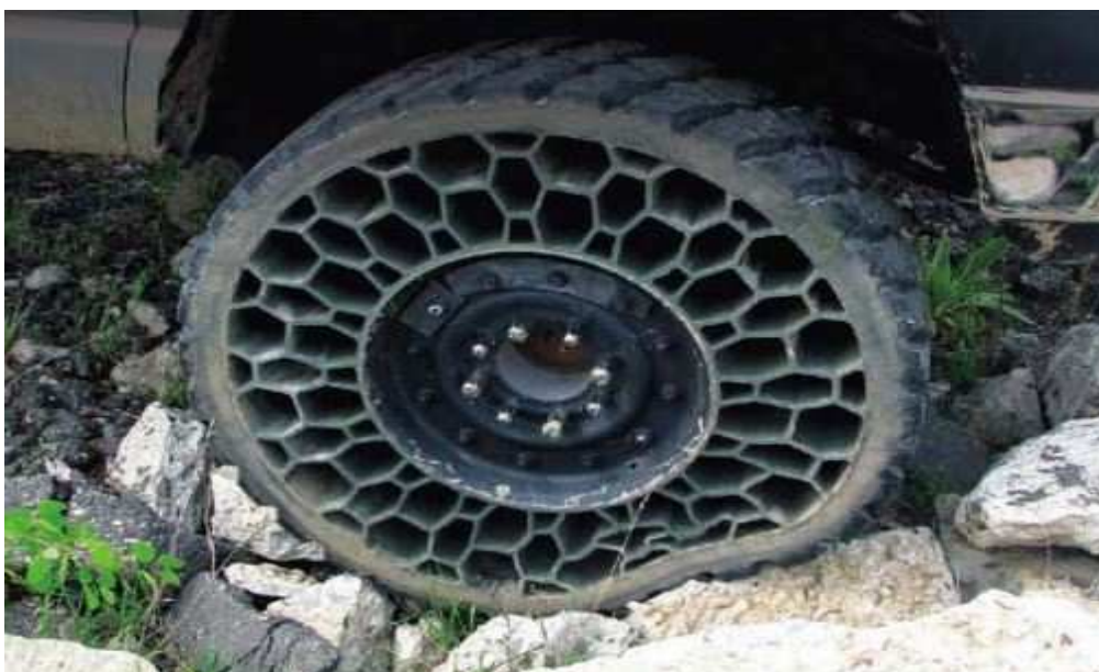
Fig. 2.1.1.1. Non-pneumatic tire and conditions in which copes [II]
