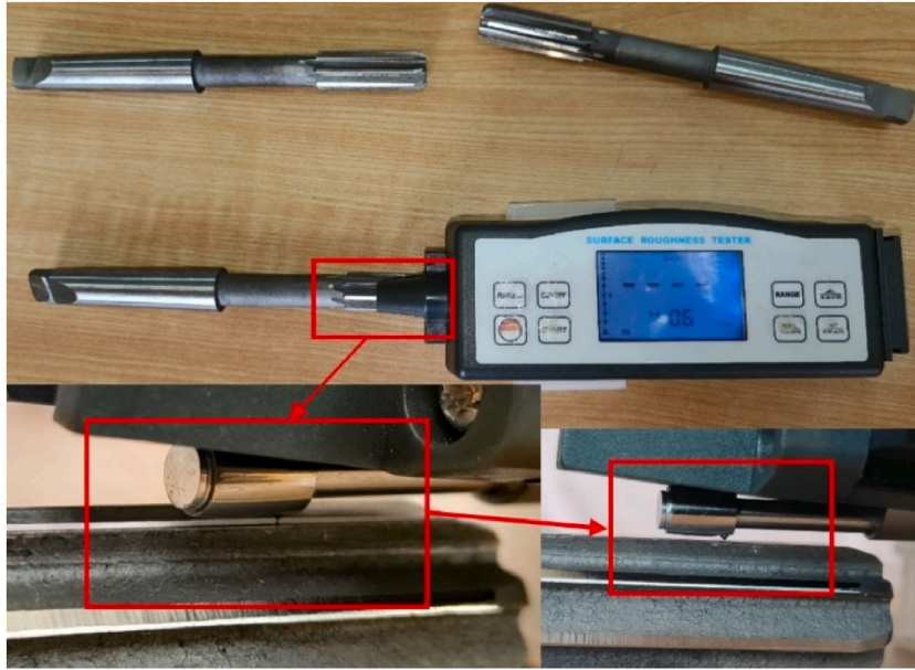
Fig. 1. Measurement process of surface roughness (Ra and Rz) on specimens.
