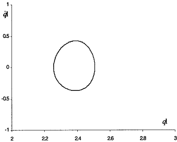
Fig. 8. Phase plane \{q_1, \dot{q}_1\} trajectory for the 3R-robot joint 1 under OLM method at r=1 , \rho=0.1 , dim=1 .
