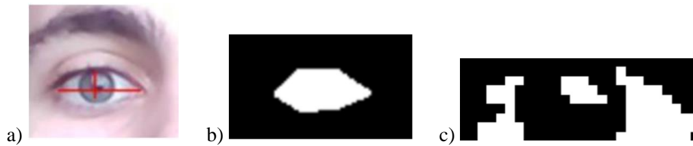
Fig. 2. Examples of eye image with height and width estimation (left), eye segmentation mask (center), and gaze estimation (right) cases. (Different scaling levels are used for the sake of easier process explanation.)
