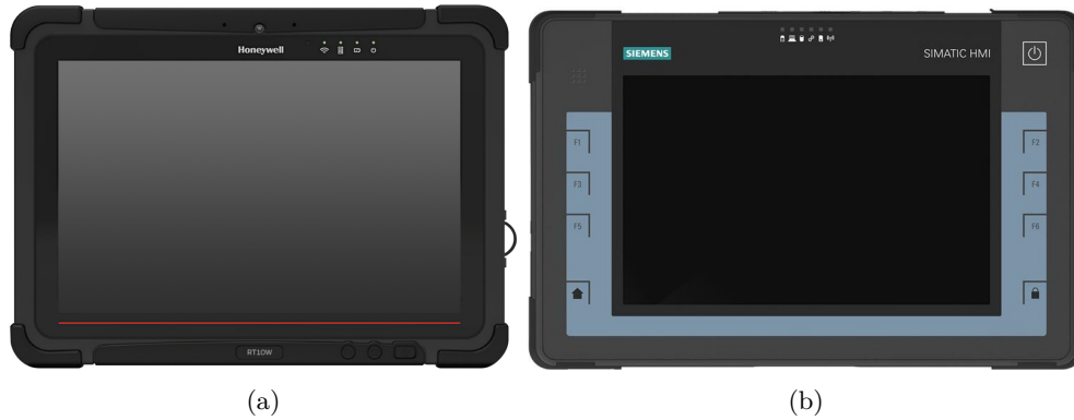
Figure 4.18: Industrial tablets: (a) Honeywell RT10W [75] and (b) Siemens ITP1000 [76].
