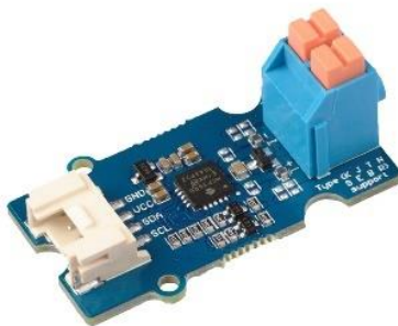
Figure 27 - Thermocouple amplifier MCP9600 [27].
