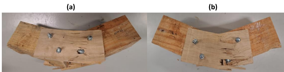
Figure 73 - First tested specimen of the bolted double strap joint (M6 bolts) front (a) and back (b) view.
