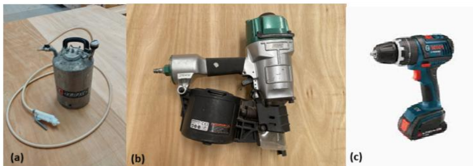
Figure 52 - pressure glue applicator (a), pneumatic coil nailer (b), and drill (c).
