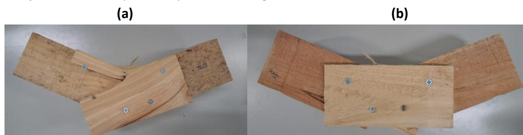
Figure 71 - First tested specimen of the fastened double strap joint (M4 fasteners) front (a) and back (b) view.
