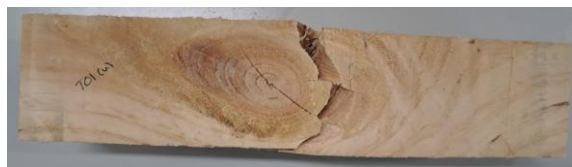
Figure 64 - Bottom view of the fourth specimen of the 80x70 mm 2 wooden beams.
