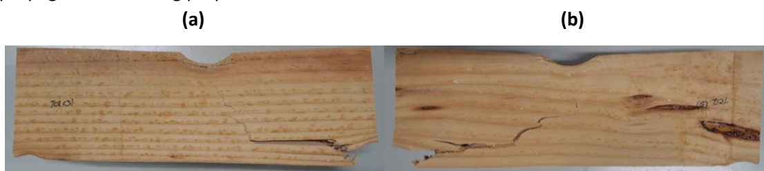
Figure 65 – First tested specimen of the 100x80 mm 2 wooden beams front (a) and back (b) view.
