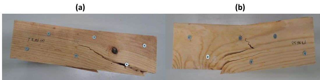
Figure 75 - First tested specimen of the double strap joint with chamfer (M6 fasteners) front (a) and back (b) view.
