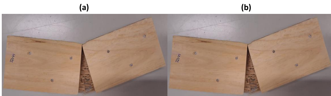
Figure 68 - First tested specimen of the laminate joint with junction alignment front (a) and back (b) view.
