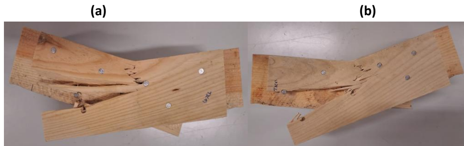
Figure 69 - First tested specimen of the double strap joint front (a) and back (b) view.
