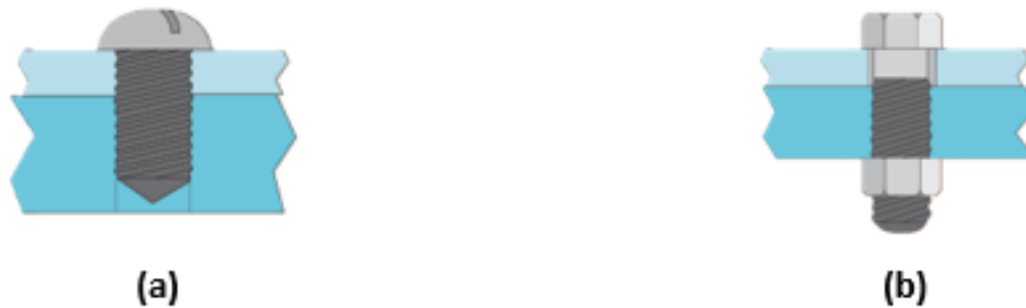
Figure 17 - bolted connection using a nut (a) Bolted connection fasteners in a part (b) (adapted from [45]).
