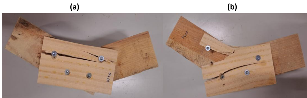
Figure 72 - First tested specimen of the fastened double strap joint (M6 fasteners) front (a) and back (b) view.
