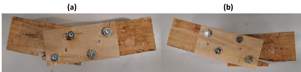
Figure 74 - Second tested specimen of the bolted double strap joint (M10 bolts) front (a) and back (b) view.
