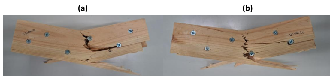
Figure 76 - First tested specimen of the double strap joint with chamfer (M6 fasteners) front (a) and back (b) view.
