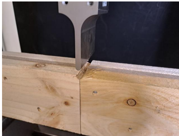
Figure 61 - Penetration of the punch in the wood.
