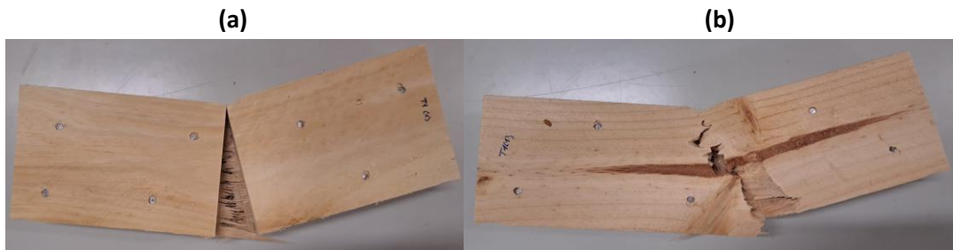
Figure 66 - First tested specimen of the simple laminate joint front (a) and back (b) view.
