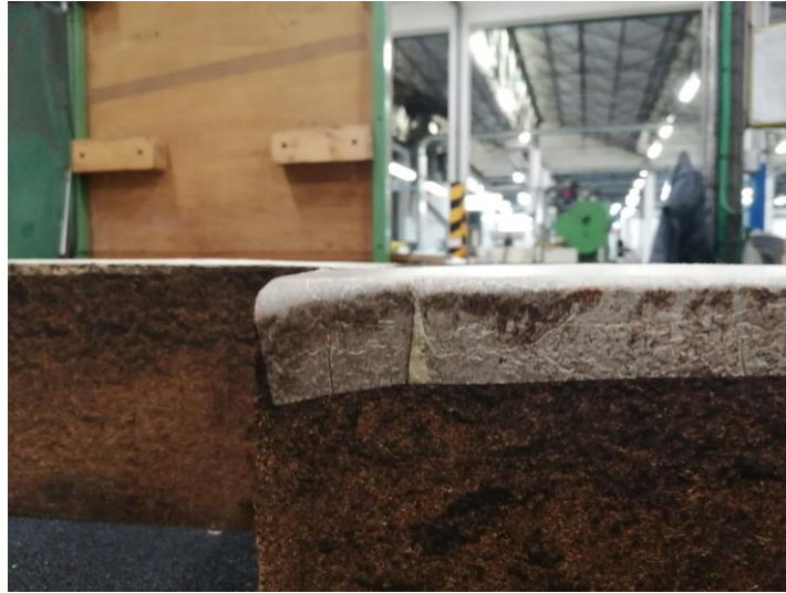
Figure 47 - Condition of the blocks using damaged molds 1.
