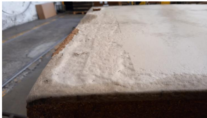
Figure 48 - Condition of the blocks using damaged molds 2.
