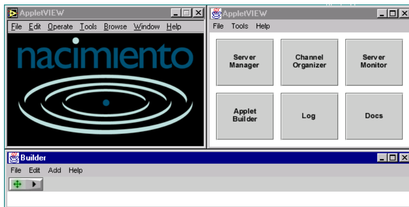
Figure 4: Print-Screen of AppletView acting as the Web server (top right) after creating the Java-based interface of a given VI (bottom).
