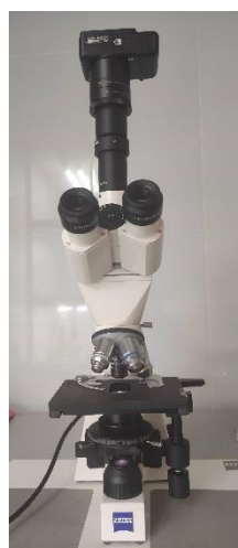
Figure 6| Optical microscope coupled to the digital camera for photograph and video recording to assess morphophysiological parameters using specific software.
