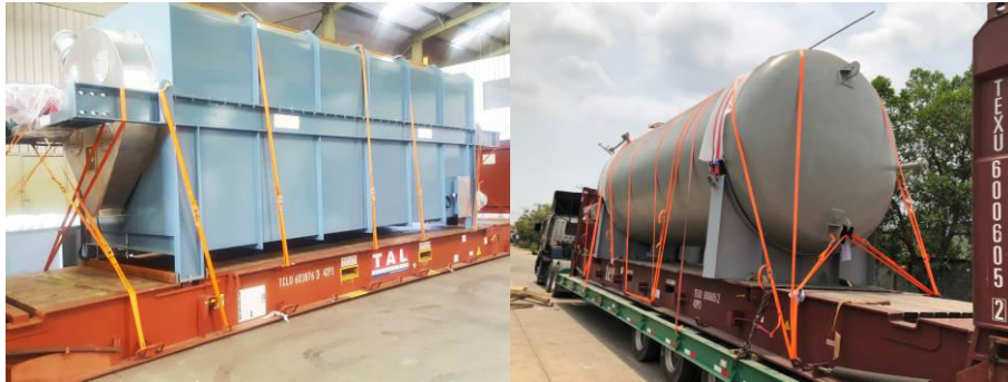
Figure 92 - Example of fifth load case (lashing with straps) [90, 115].
