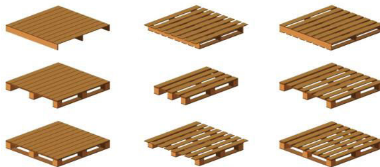
Figure 10 - Different wood pallet designs (adapted from [14]).
