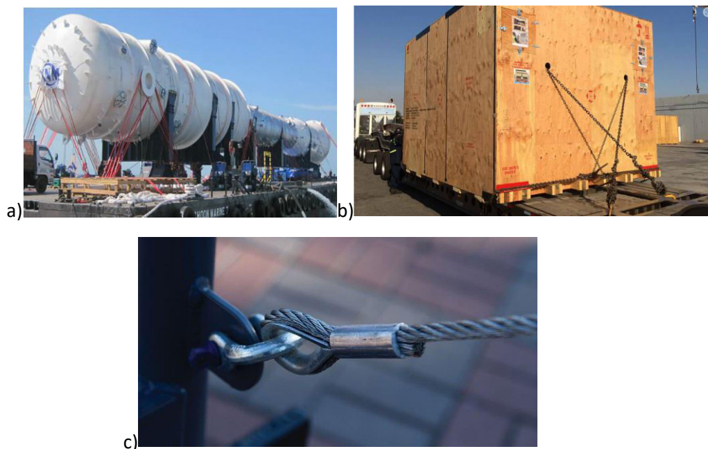
Figure 31 - Lashing solutions: webbing straps [86] (a), chains [84] (b) , and steel wire ropes [92] (c).
