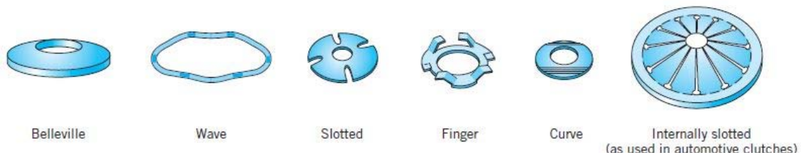
Figure 26 – Types of spring washers (Juvinall & Marshek, 2012)
