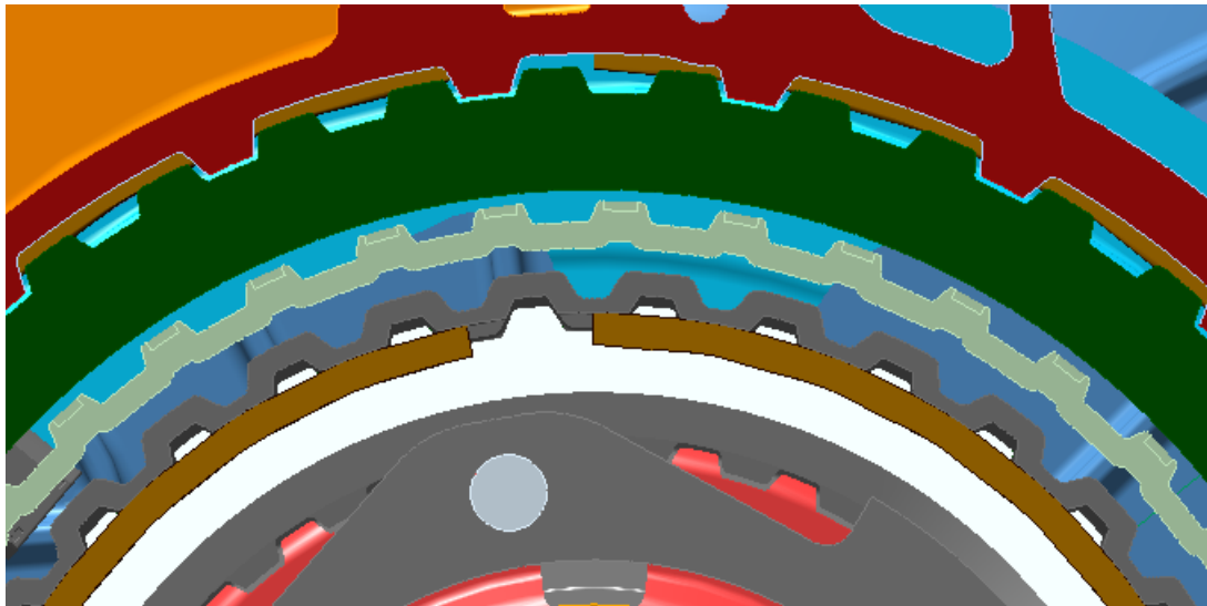
Figure 72 - Spline matching between endplate reverse clutch and transmission housing (courtesy of Punch Powertrain NV)
