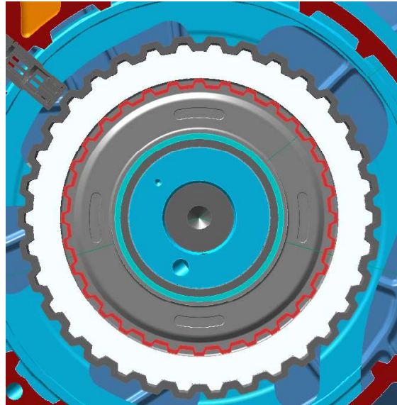
Figure 63 - Splines matching between the FWD separator plate (white) and the CC (black) (courtesy of Punch Powertrain NV)
