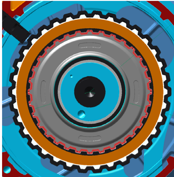
Figure 65 – Matching between sun gear (red) and clutch plates (courtesy of Punch Powertrain NV)
