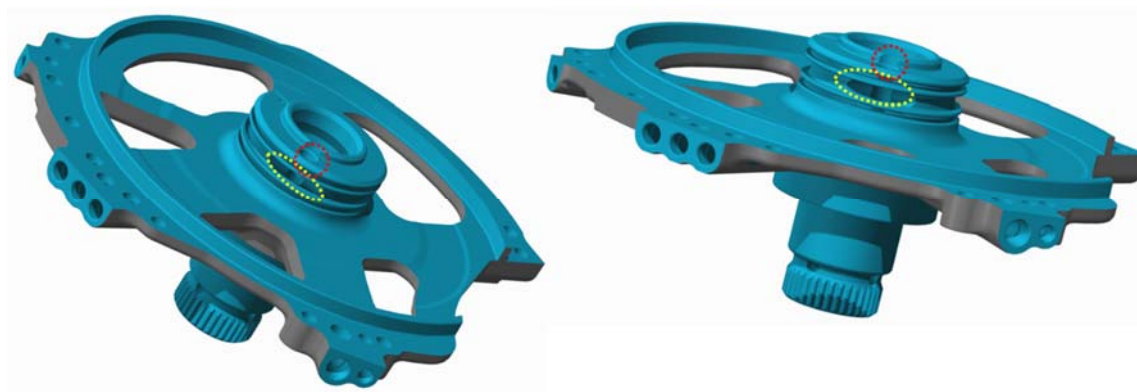
Figure 113 – Stator plate's channels for forward clutch oil circuit (courtesy of Punch Powertrain NV)
