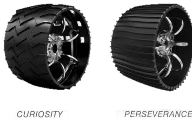
Figure 11. Comparison between Curiosity and Perseverance wheels [23]
