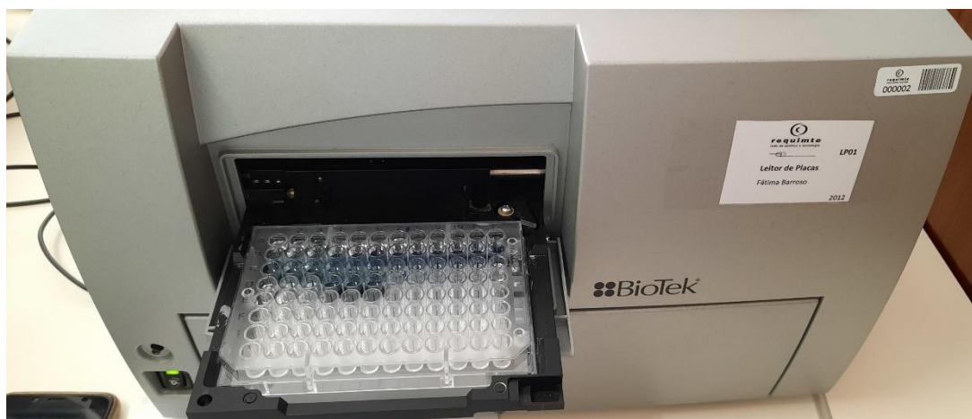
Figura 3.2 - Leitor de microplacas Multi Mode Microplate Reader with Gen5 2.0 software (BioTek Instruments, USA).
