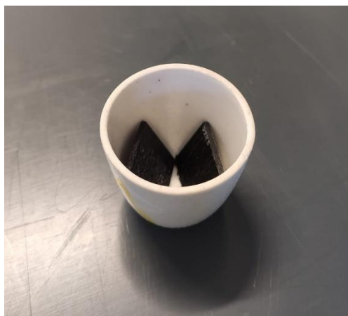
Figure 37 – Crucible with sample before incineration
