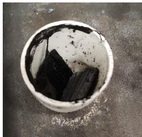
Figure 38 – Crucible with sample after incineration
