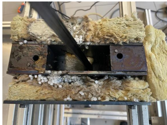
Figure 22 – Molten polymer inside the polymer pool
