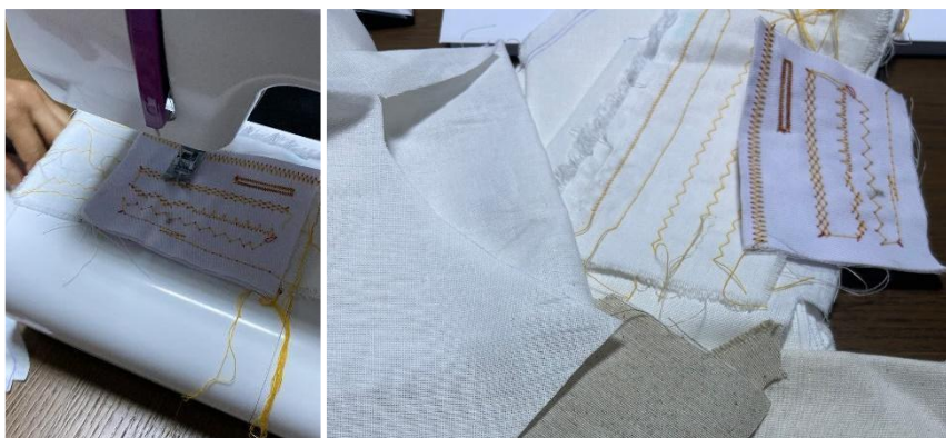
Figure 9 Stitching test showing various stitch patterns exploration suitable for application on the BioMask sandwich material.
