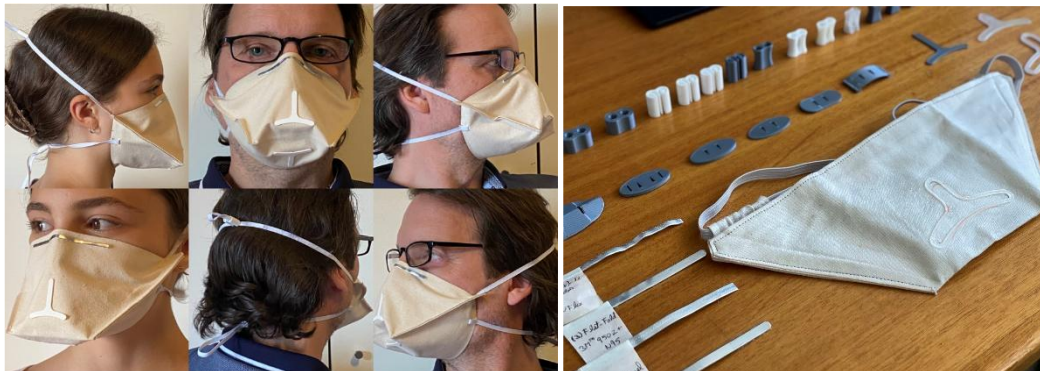
Figure 8 Human head size variation evaluation and 3D printed accessories development, including a removable metal nose clip.
