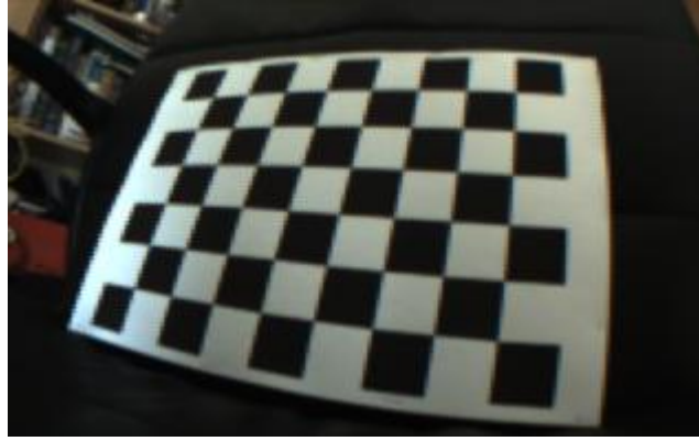
Figure 10 Checkboard used for calibration. Image captured by a Pixy camera where there is easily seen the camera distortion.
