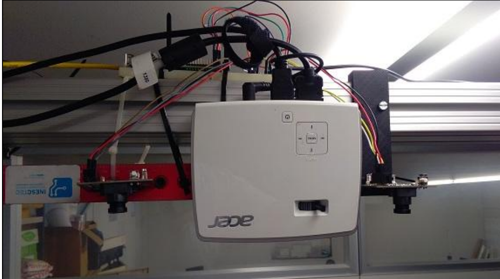
Figure 32 Setup where the cameras are mounted above the working area. It can be seen the left and the right camera and a projector in middle. The computer is above the rail.
