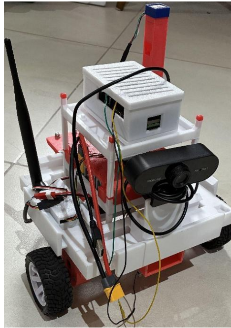
Figure 7. X-Lakbay snap-fit 3D-printed robotic platform [22]. Cropped from Esquivias et al. (2025), Figure 1A, under the Creative Commons Attribution Licence.
