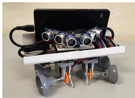
(b) Andruino-R2 robotic platform integrating an Android phone. Cropped from Lopez-Rodriguez and Cuesta (2021) , Figure 1, under the Creative Commons Attribution Licence (CC BY).
