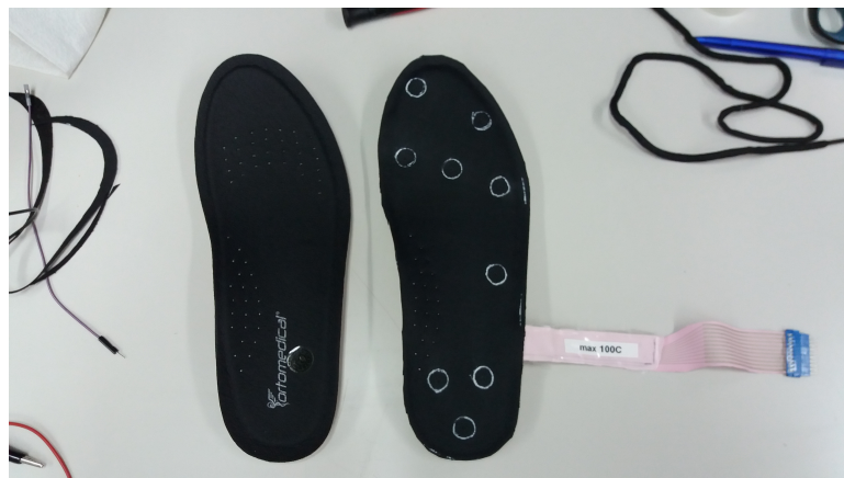
Figure 3.6: Integration of insole into the diabetic shoe
