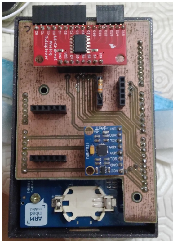
Figure 3.13: Final monitoring system - PCB coupled to the micro-controller
