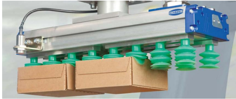
Figure 10 - Vacuum gripper grasping cardboard boxes (Schmalz, 2015)
