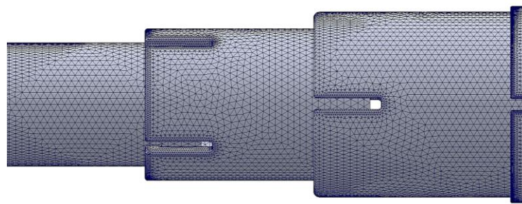
Figure 80 - Details of the mesh used in the grippers structure simulation
