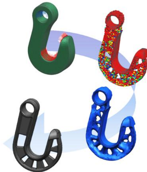
Figure 21 - Evolution of a model using NX CAE software (NX, 2011)
