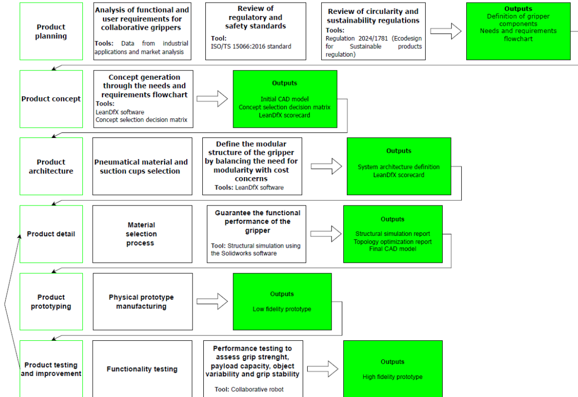
Figure 22 - Collaborative robotic gripper development methodology
