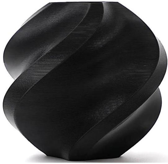
Figure 36 - Representative component fabricated using Bambu Lab PLA basic (Bambu Lab, 2025d)
