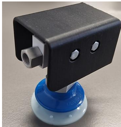
Figure 89 - Suction cup mount, vacuum generator, and suction cup assembly
