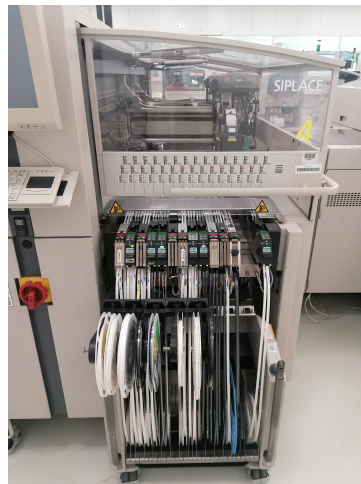
Figura 4.5: Máquina Pick and Place .
