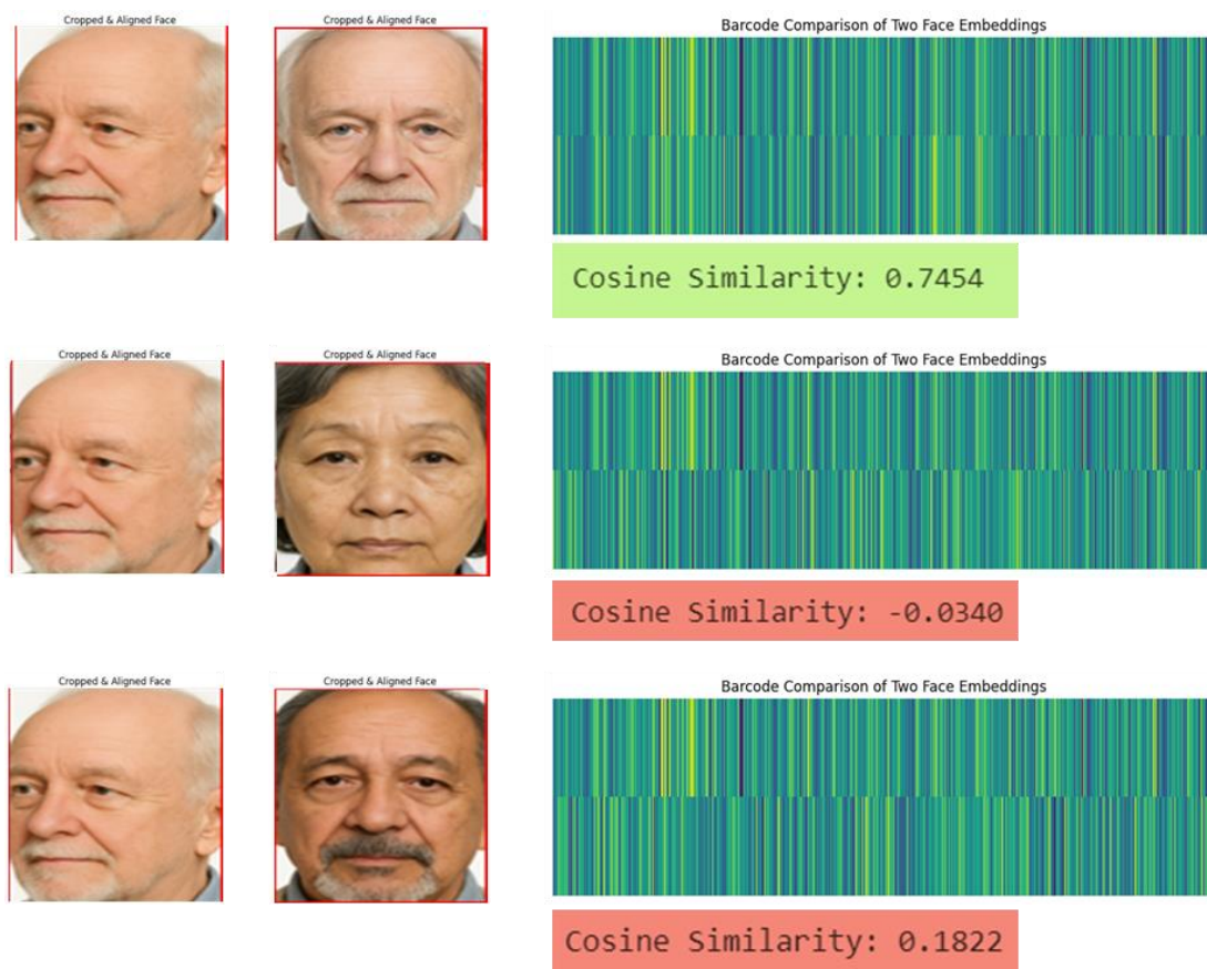
Figure 18 – Face recognition results using cosine similarity between embeddings.
