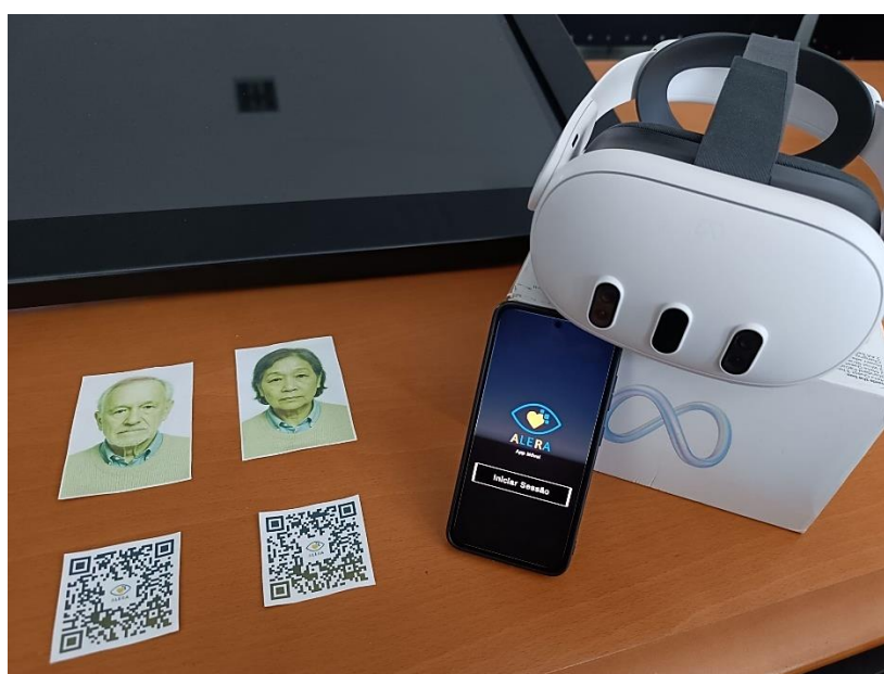
Figure 23 – Apparatus used for the case study. From left to right: QR codes and patient photos, Samsung Galaxy S23 running the AleRa companion app, and Meta Quest 3 headset equipped with the Elite Strap accessory.
