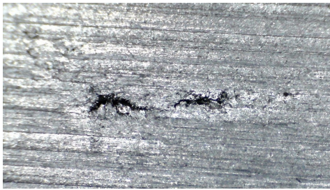
Figure 36 – Microscopic view of lunker defect.
