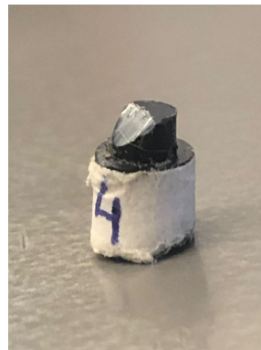
Figure 78 – Pin after 900 seconds of test.
