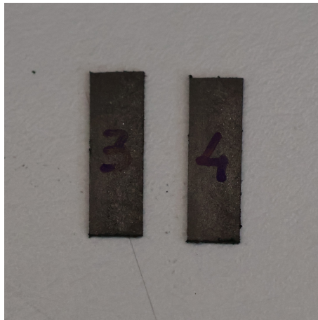
Figure 28 – Prepared specimens for DMA testing.
