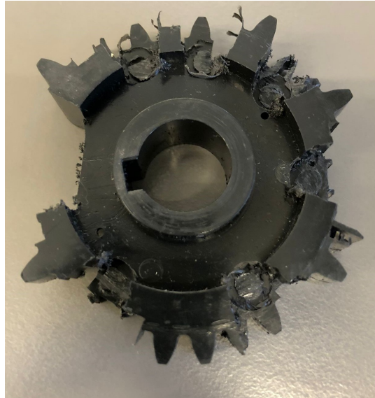
Figure 32 – POM machined gear.
