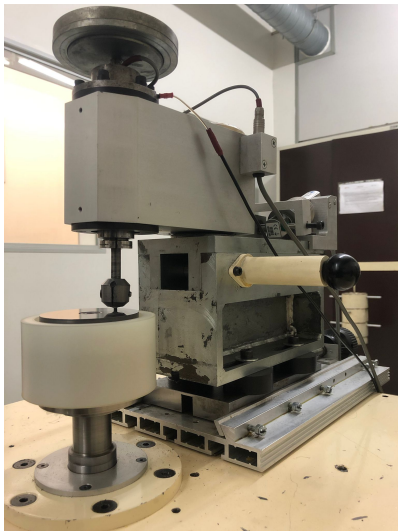
(a) Pin-on-Disc setup.
