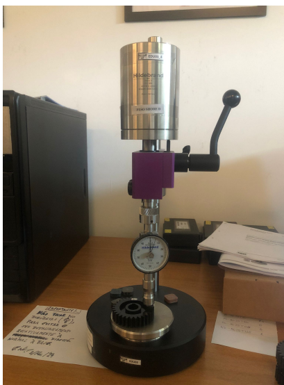
(a) Hardness Shore D setup.
