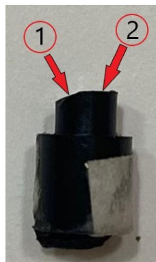
Figure 82 – Final shape observed in pins after testing.
