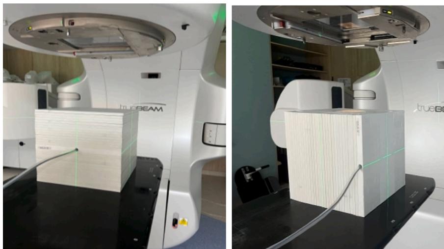
Fig. 1. Positioning of water or tissue equivalent slab phantom (here: PTW RW3) and Farmer type ionisation chamber at the isocentre of the kV CBCT On-Board Imager on a Varian Truebeam linac. Left: Farmer chamber in the central position to measure CBDI_{c,f}(slab) . Right: Farmer chamber in the right peripheral position to measure one of the four CBDI_{p,i}(slab) values.
