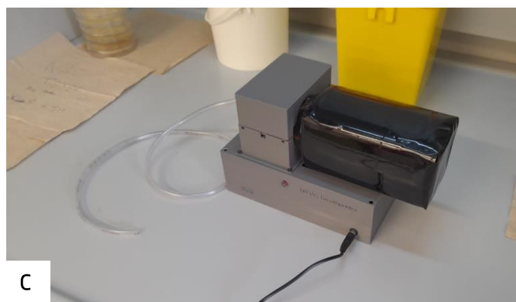
Figure 5: A and B - Function of the electronic nose used to detect the volatilome of fungi. C - Electronic nose MIDAS Breathprinter.
