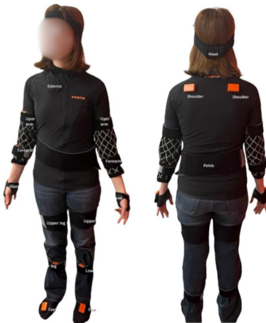
FIGURE 1 Placement of the straps and inertial sensors of the Xsens MVN.
