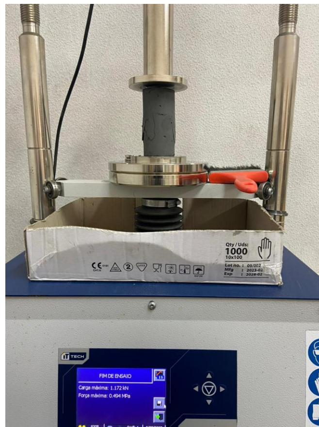
Figura 27 – Prensa S205N Unitronic (50kN).
