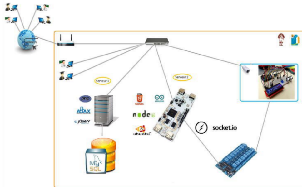
Figure 2.16: E@Slab architecture version 1 [26]
