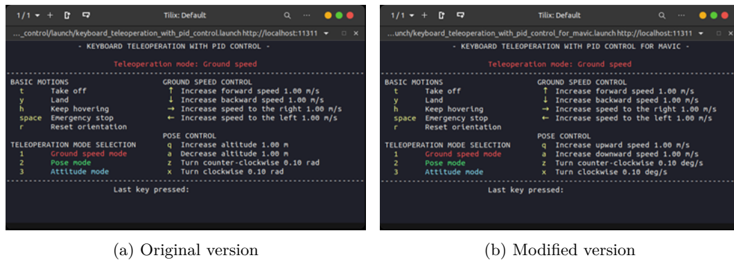
Figure 5.4: Comparison between the user interfaces for the original version of the keyboard teleoperation package (a) and the modified version used in the new implementation (b).
