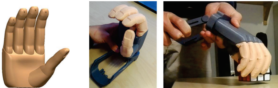
Figure 2. Functional prosthetic hand design conceived for additive manufacturing with flexible filament (TPU, Filaflex ).
