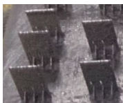
Figure 1. Ti6Al4V thin-walled plates on the building platform after SLM fabrication.
