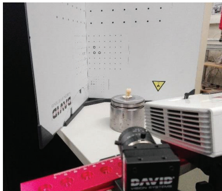
Figure 1. 3D shape acquisition of the natural tooth with DAVID System ® .
