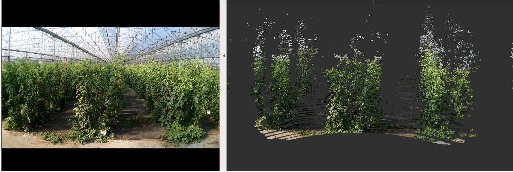
Figure 5.14: Projected XYZRGB cloud and RGB image (1920x1080) visualized in Rviz.
