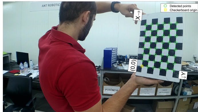
Figure 5.5: Matlab Camera Calibration corner detection - 1920x1080 image.
