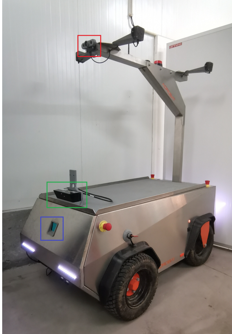
Figure 5.1: Robot with sensors used to collision avoidance highlighted.
