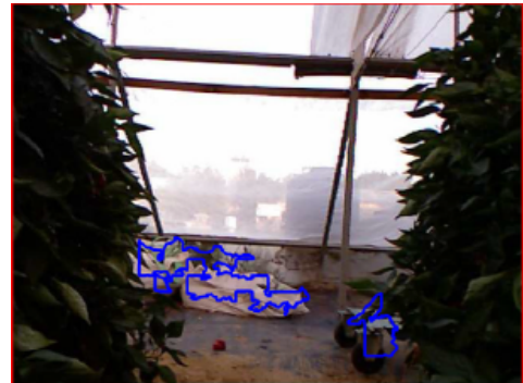
Figure 2.3: Detection based on color classification [24].
