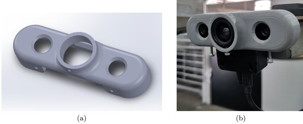
Figure 5.3: 3D modeled support: (a); Support and lens attached to the camera (b).
