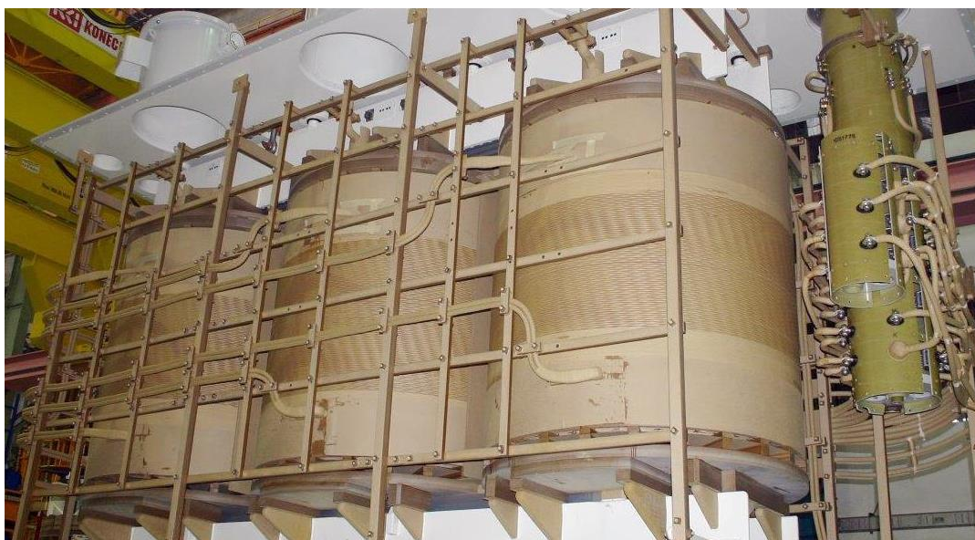
Figure 3 - Transformer active part isolated with Kraft paper
