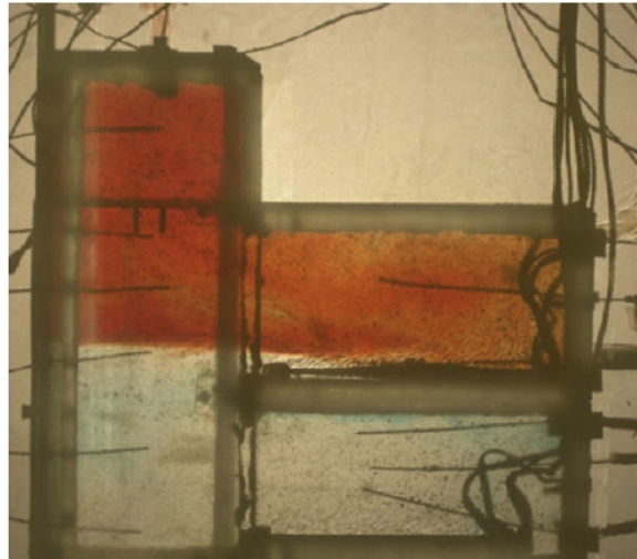
Figure 2.36: Photograph of a small-scale model filled with water for flow visualization of a two-storey building with a common atrium. Livermore and Woods (2007)
