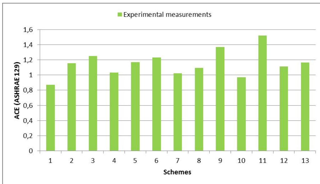
Figure 5.8: ACE (ASHRAE 129 method) experimental results
