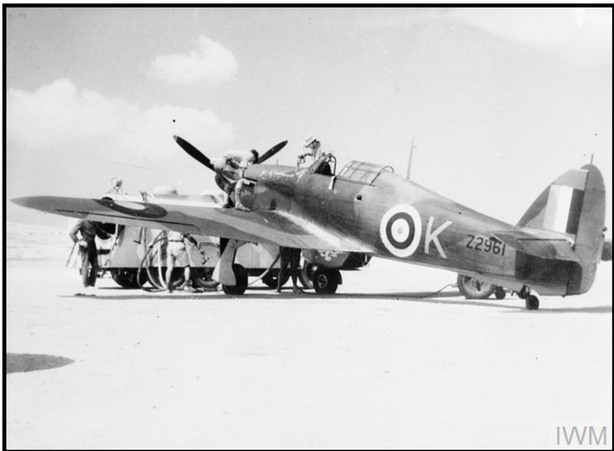
Fig. 403 Hawker Hurricane Mark IIA, Z2961 'K', of the Malta Night Fighter Unit being refuelled and re-armed at Ta Kali, Malta.
