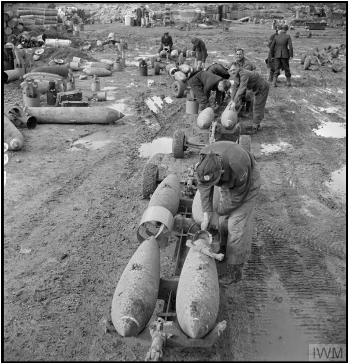
Fig. 424 RAF armourers, assisted by soldiers, fit tail fins to 500-lb GP bombs on trolleys at Luqa, Malta, before they are towed to Vickers Wellingtons for a raid on Axis forces in North Africa. Fonte: https://www.iwm.org.uk/collections/item/object/205212165
