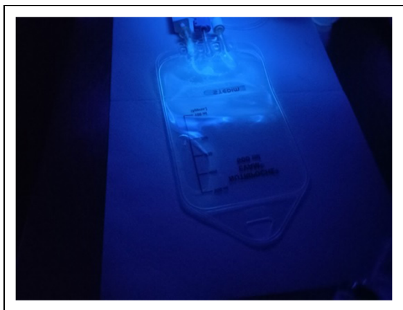
Figure 2. Positive control obtained by applying ultraviolet (UV) light in an intravenous fluid administration bag containing tonic water.
