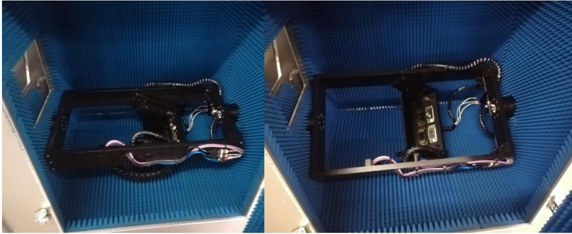
Figure 27 Rotatory plates inside the anechoic chamber.
