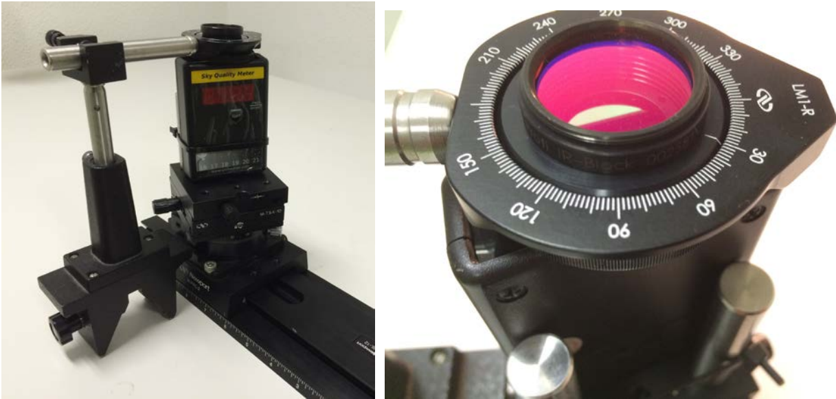
Figure 1. (Left) SQM-L on a rotation stage with linear displacement platforms. The polarizer and the IR blocking filter are located just above the detector. (Right) Polarizer and IR blocking filter.
