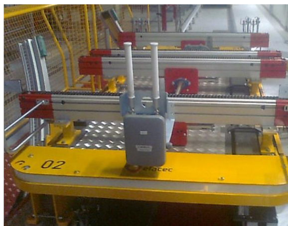
Figura 23 – Cliente Wireless Ethernet
