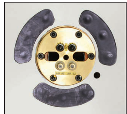
Utility connections at faceplate
