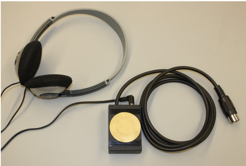
Figura 2.20 - Monitor de sons cardíacos HSM-300. [22]
