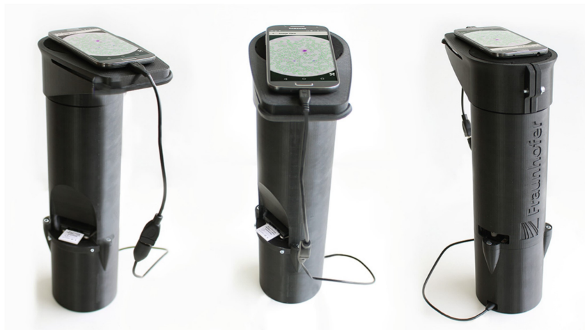
Figure 4.1: The \mu SmartScope prototype, with smartphone attached and microscopic slide inserted [4].
