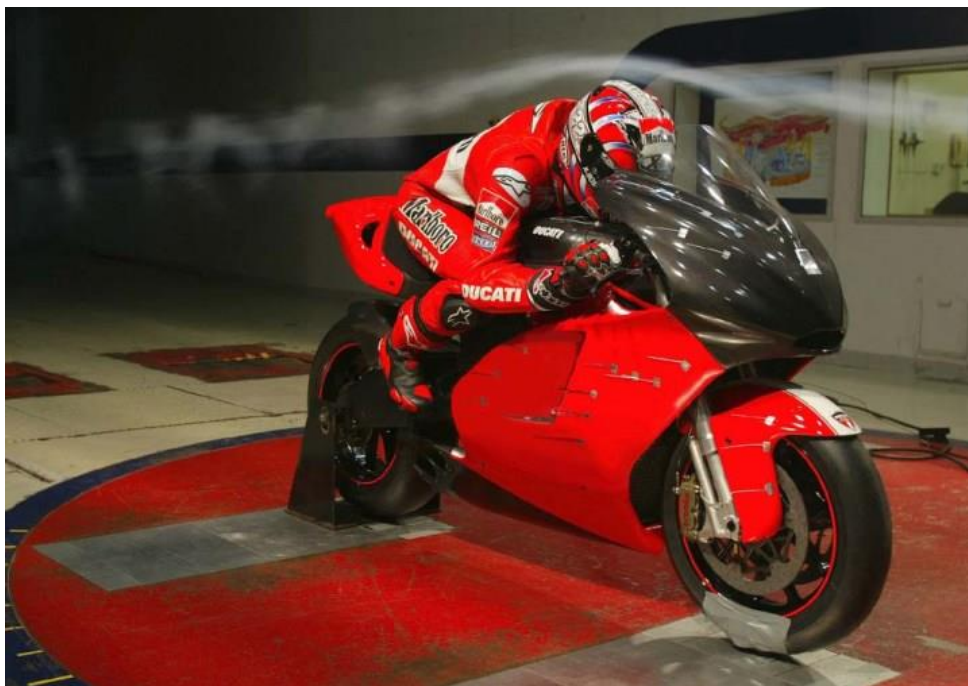
Figure 21 - Wind tunnel testing of a Ducati GP motorcycle (Guide, 2016)
