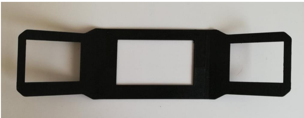
Figure 92 - 3D printed front frame scale model (front view)
