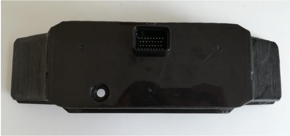
Figure 91 - 3D printed rear cover scale model (rear view)
