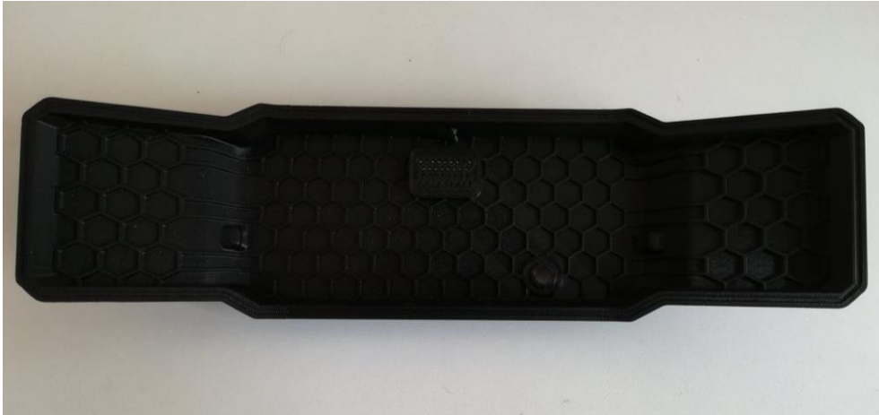
Figure 89 - 3D printed rear cover scale model (front view)
