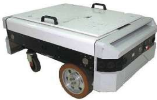
Figure 1 – Robuter Mobile Platform
