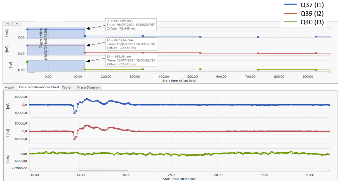
Figure 58 Anomaly detection at 200 ms acquisition rate with waveform record.
