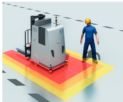
(a) Laser ranging based on the time of flight principle [53]. (b) Mobile hazardous area protection via ESPE devices [40].
