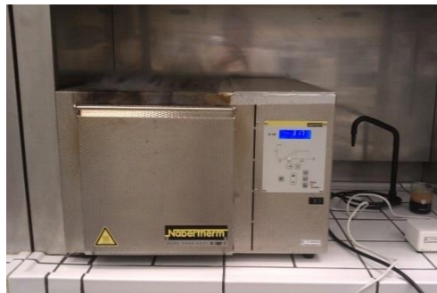
Figura 3.2 - Mufla (B 150, NABERTHERM).
