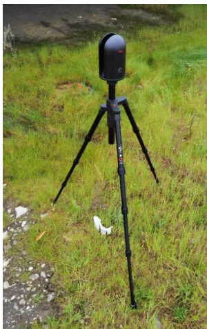
a) Pormenor do laser scanner
