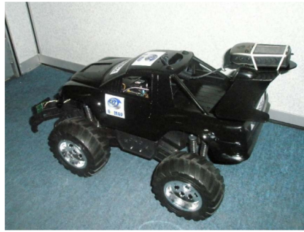
Figura 3.6: RC Truck com GPS e Sonar [18]
