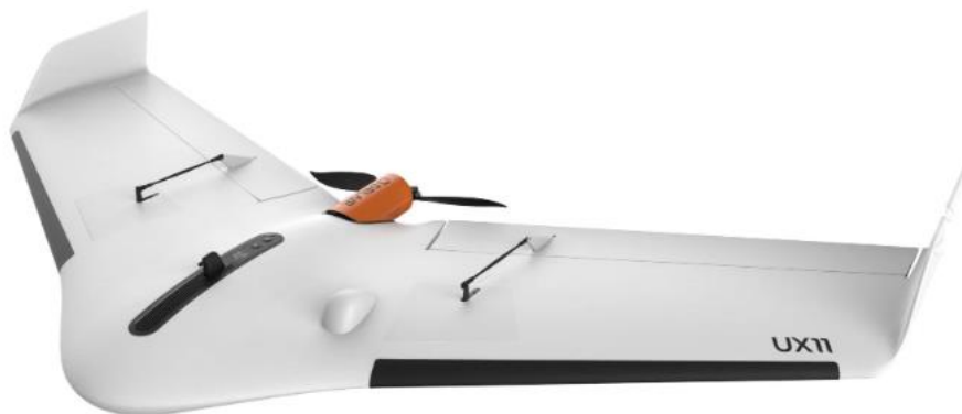
Figura 30 – Delair UX11: UAV de asa fixa [34]
