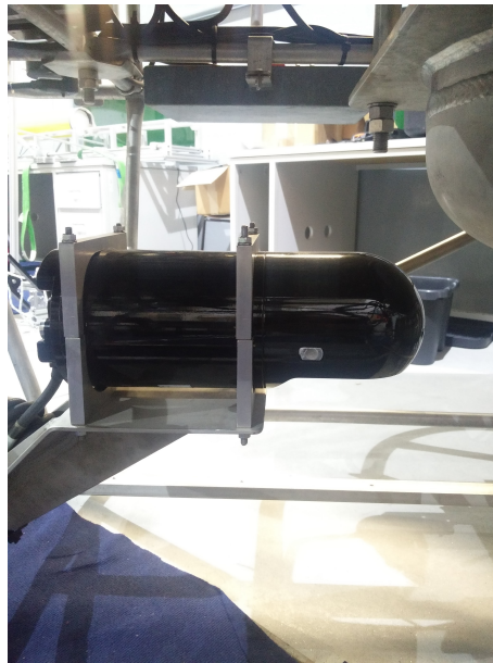
Figura 4.18: DVL Teledyne Explored Phased Array SelfContained .
